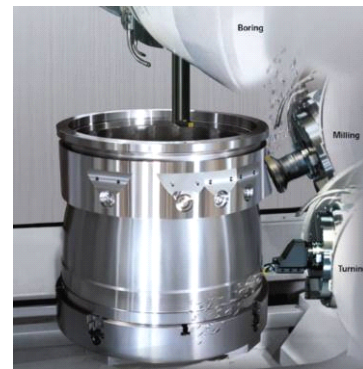
Figure 5: Examples of machining by multi-tasking machine tool (Machining center-based).
