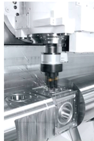
Figure 9: Boring by U-axis tool (D'andrea TA-C160)
