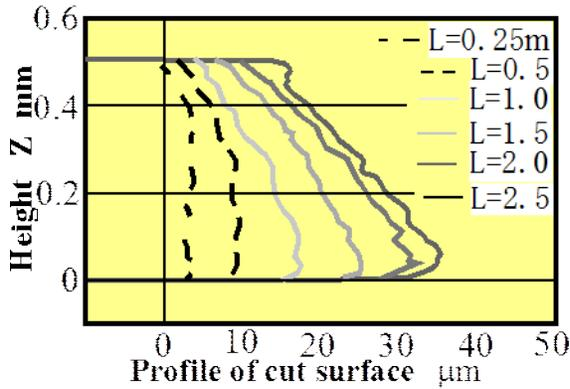
Figure 8: Changes in shape of side face caused by tool wear
