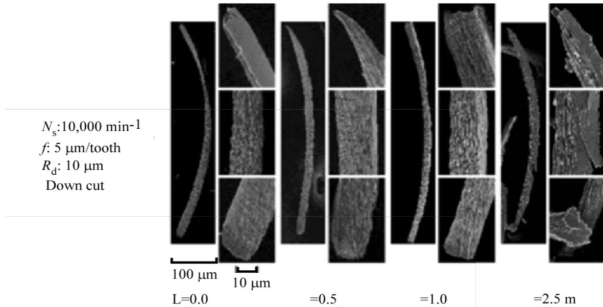
Figure 13: SEM photos of chips
