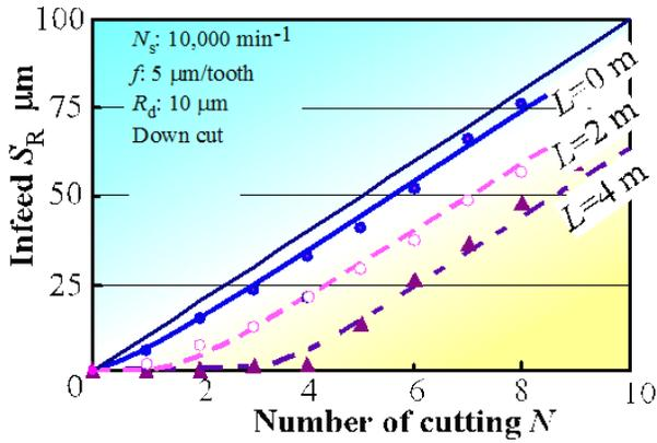
Figure 7: Infeed and changes in residual stock removal
