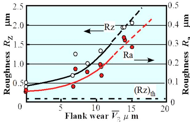
Figure 14: Relationship between surface roughness and average flank wear width
