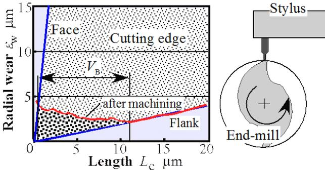
Figure 4: Measuring method of tool wear
