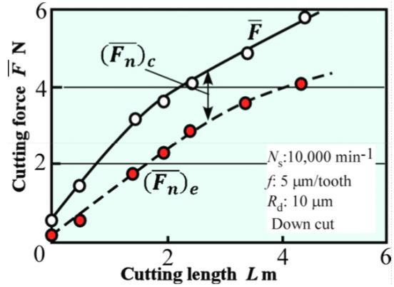
Figure 9: Separating normal force into elastic contact force and normal cutting force
