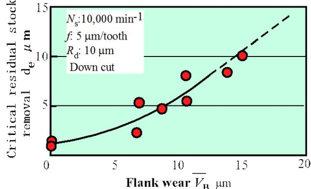
Figure 11: Critical residual stock removal and average flank wear
