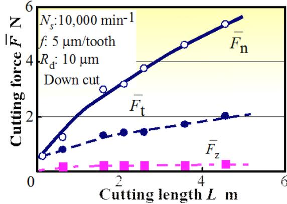
Figure 6: Changes in average cutting resistance depending on cutting length
