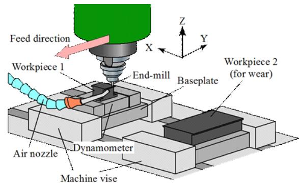
Figure 1: Schematic diagram of experimental set up
