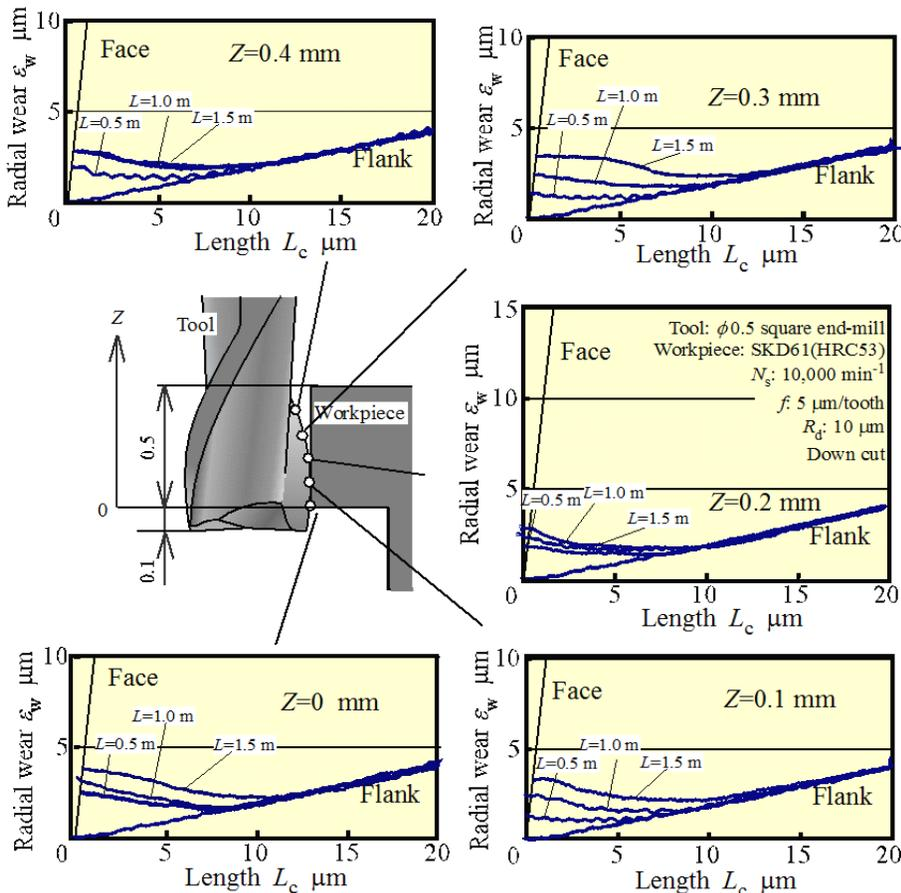
Figure 12: Cutting length and flank wear width in the Z-axis direction
