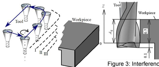
Figure 2: Machining paths to analyze cutting phenomena
