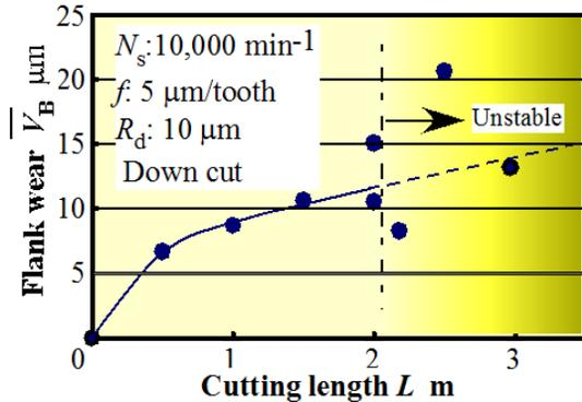
Figure 10: Average flank wear width with cutting length
