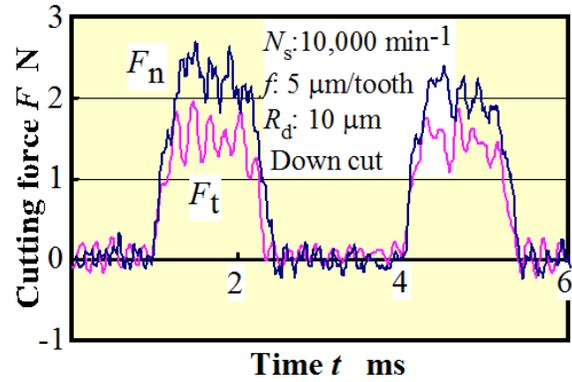
Figure 5: Changes in cutting resistance during a rotation
